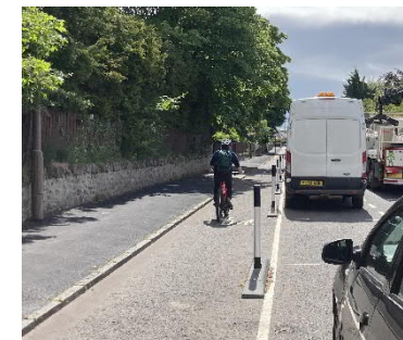
Figure 6.1: With-flow light segregated cycleway example
